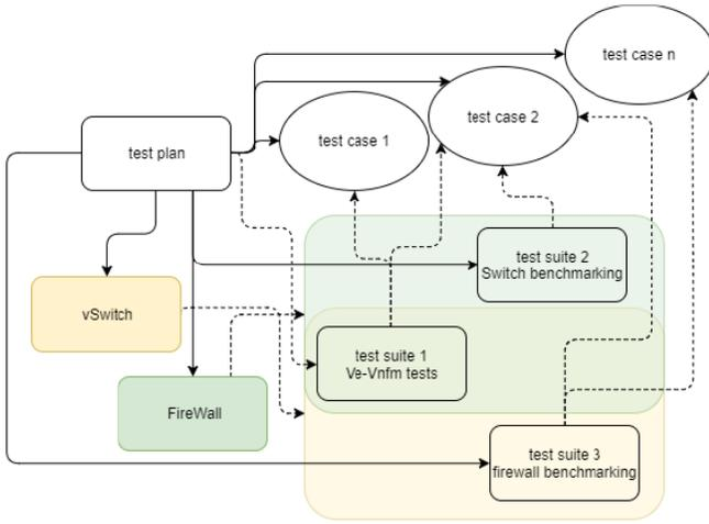
Fig. 2. Test plan, test profile, test suite and test case
